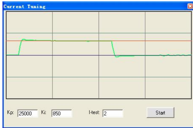
Figure 29: Step response with better K_p and K_i of current-loop( K_p=25000, K_i=850 )
