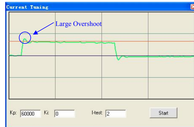
Figure 28: Response with High K_p of current-loop ( K_p = 60000 )
