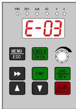
Fig.3—5 Alarming display status
